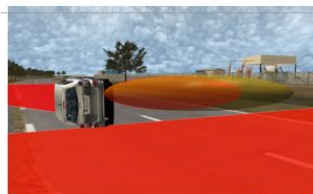
TPRD release on tilted vehicle
