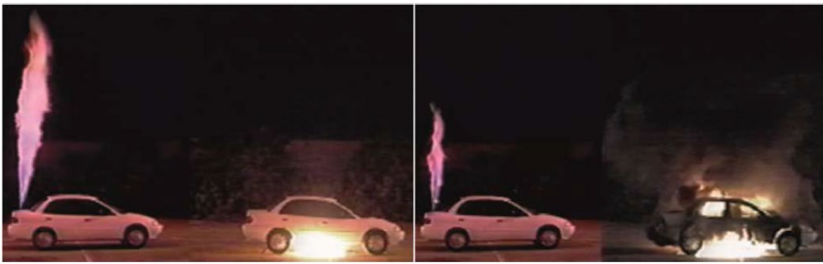
Figure 3. Hydrogen jet fire and gasoline fire: 3 s (left) and 60 s (right) after a car fire initiation [13].
