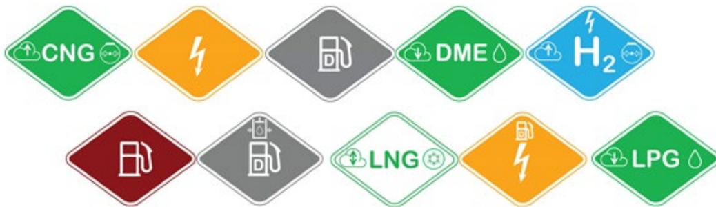
Figure 2. Colours and symbols suggested by CTIF for the development of standardized signs
