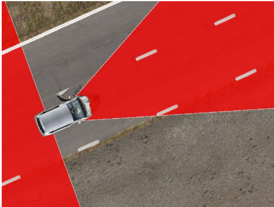
Figure 43 : (In red) forbidden angles for reaching a FCH car in fire on wheels. ©Crise-2015
