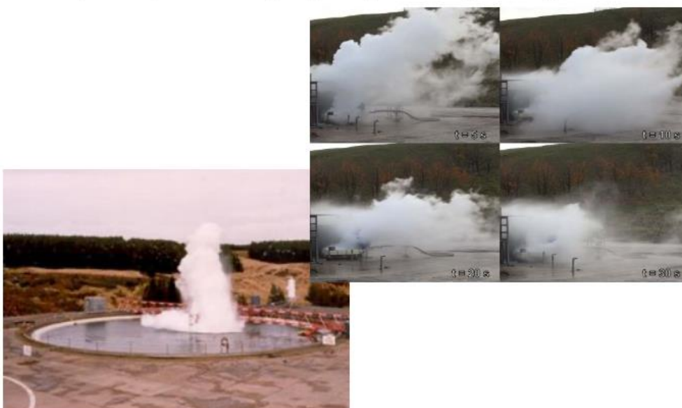
Figure 5: Rapid Phase Transition representation. Source Air Liquide Image Bank
