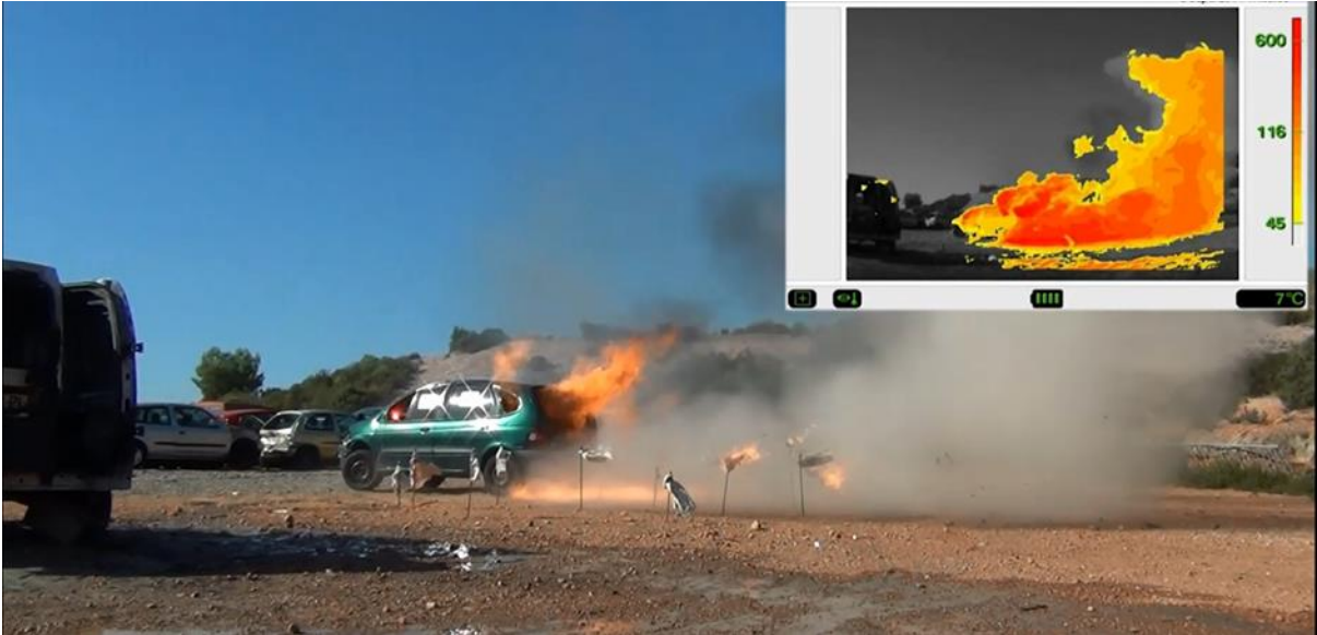
Figure 8 : H2 tank fire (700b) (ENSOSP 2014).
