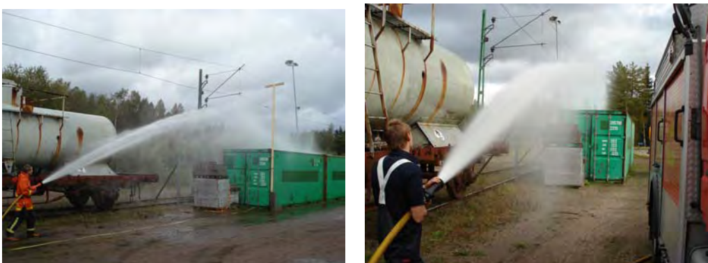
Figure 5.1 Experimental set-up and tests for the discharge test using firefighting nozzle.
